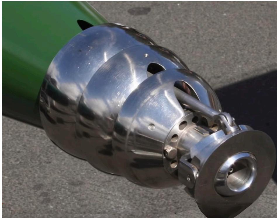
Adjustable by means of simple actuators it allows the flow of gas injected on one side or the other of the torpedo to be modulated. This creates a differential friction on opposite walls and thus represents an extremely effective means of piloting the machine, fundamentally different from the classic ailerons, or the swivel nozzle system.
