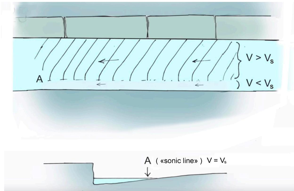
*Water flow in the gutter, bird's eye view.*
