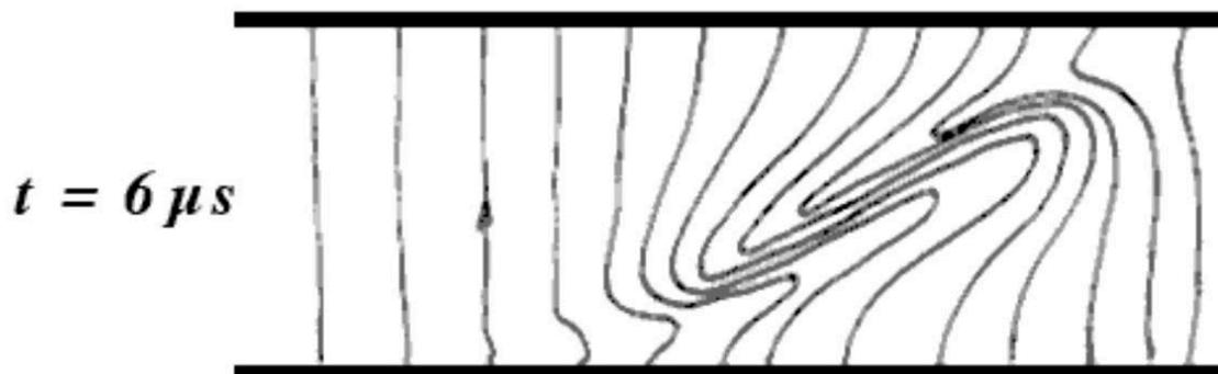
Distortion of the electric current lines by the electrothermal instability of Velikhov
