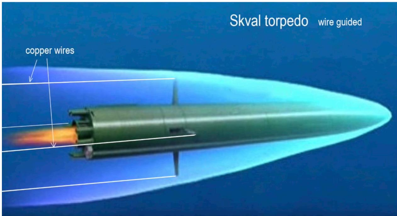
Hereafter, its nozzle of injection of the gas resulting from the combustion of a solid propellant:
