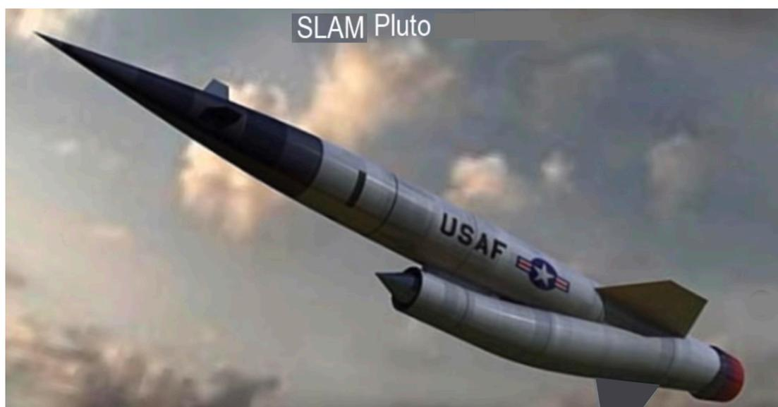
It is then a heavy cruise missile, evolving at low altitude at Mach 3. It is equipped with a thermopropulsive nozzle, a kind of ramjet where the air is brought to 1200° after passing through a hundred tubes ensuring the cooling of a mini nuclear reactor, without any armour. It is represented installed on a platform mounted on rails. It is then propelled by powder boosters before its nuclear engine enters in action. Hereafter the nuclear engine of Pluto:
